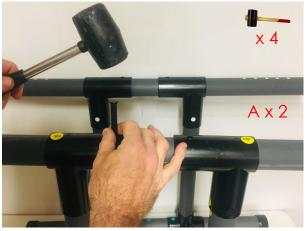
6) Slide the Frame Rails (A) through the Cut T's.
